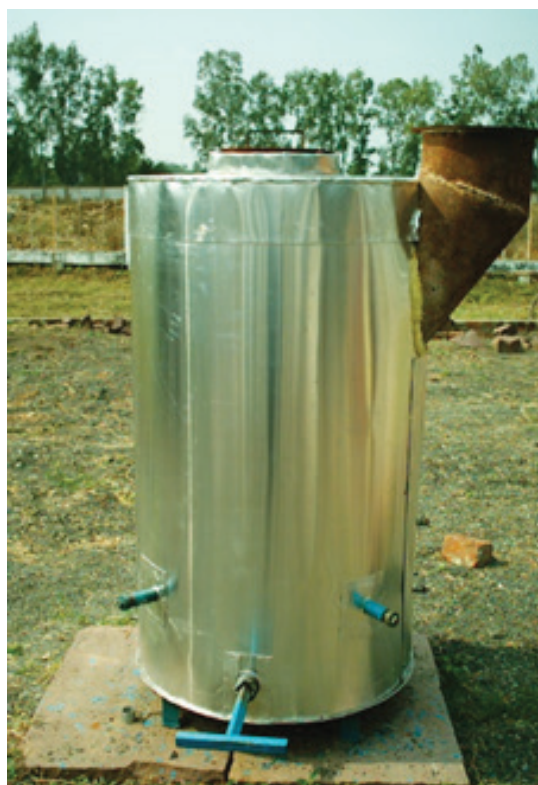
Figure 4. CIAE 100 kW natural draft gasifier
