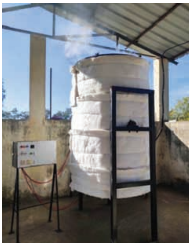
Figure 6: Electrically controlled torrefaction system developed by CIAE, Bhopal
