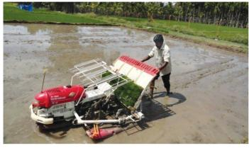
Fig. 1. Self propelled walk behind rice transplanter (kukje) in operation
