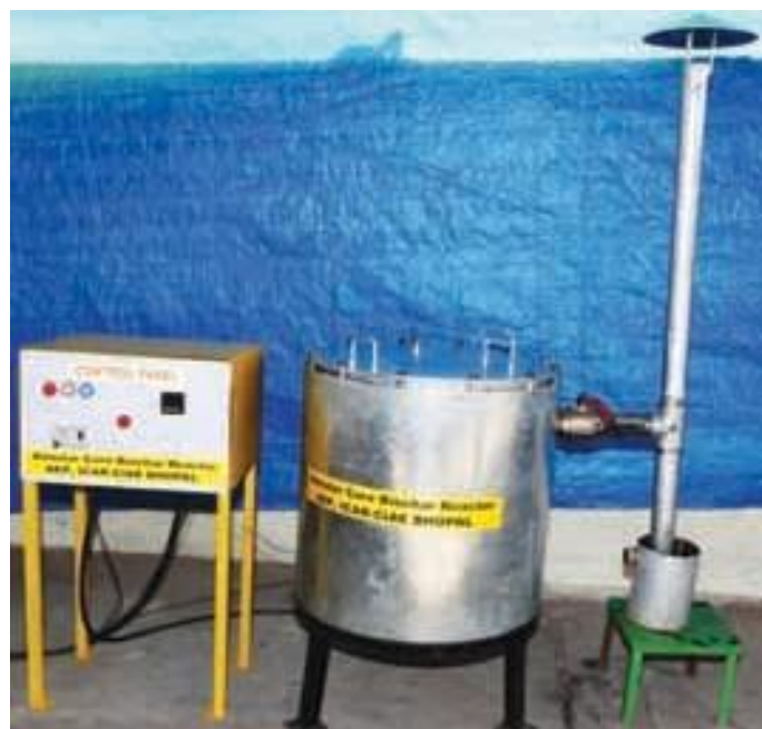
Figure 5. Annual core biochar production system developed by CIAE, Bhopal
