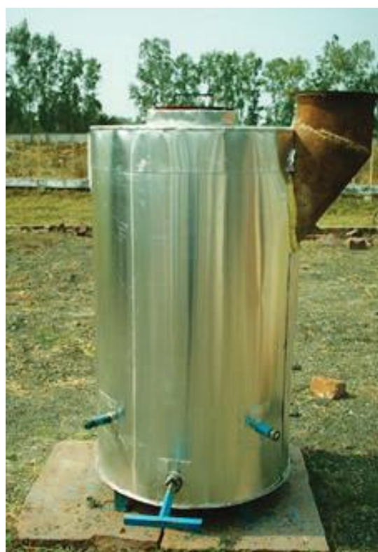
Figure 4. CIAE 100 kW natural draft gasifier
